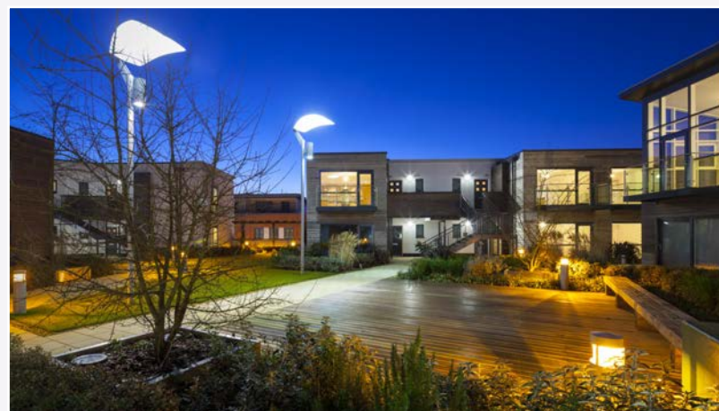
Carefully integrated lighting will create safe, attractive and usable public spaces in conjunction with the location of other furniture and planting. Light fittings should minimise light spill and excess light distribution into adjacent properties and the landscape
